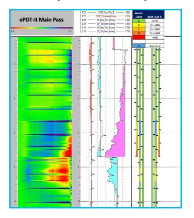
Well 2 :ePDT-II Reveals Insignificant Corrosion Damage to 30 and 20 inch casings
