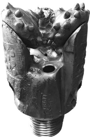
144 Scorpion Composite Plugs can be milled out with a single bit with visibly less wear than when milling out competitor plugs.
